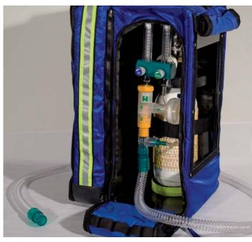
In order to administer CPAP therapy with mask or helmet without using a power source we developed a backpack that includes a 400 L oxygen supply and an high Venturi flow generator (code 9293/D)\*\* that can produce flows from 0 to 190 L/min with FiO2 adjustable from 33 to 100 %.
